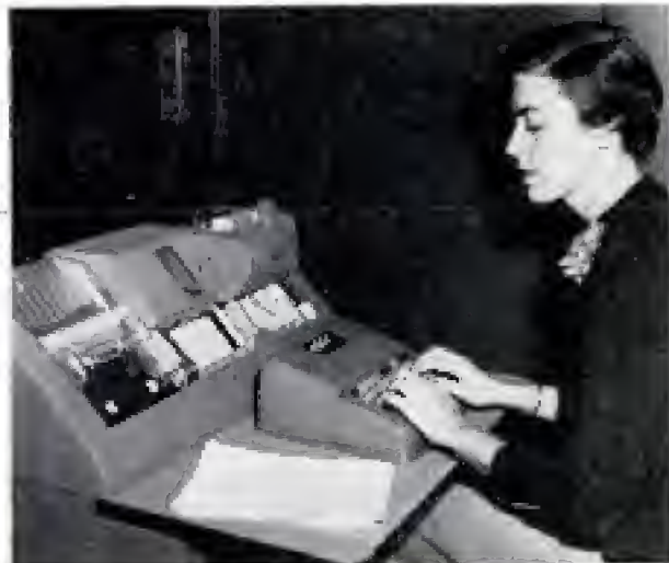
Sentences in Russian are punched on standard IBM cards for feeding into processor for translation
